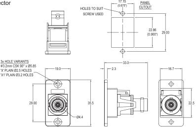
Note: Functionality is affected by cable quality, length and cable wiring configuration. Dimensions: Millimetres
