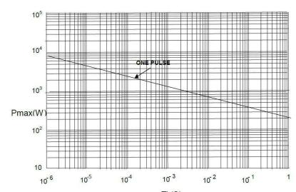
Condition test: Resistance change ≤±5% with pulse 1000 cycles as like the figure.(Reference Only)
