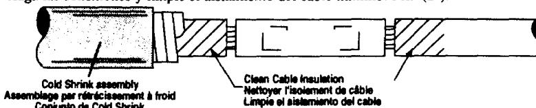
3. Locate Cold Shrink Assembly at desired starting point, position assembly 1-1/2" to 2" (3.8 to 5 cm) beyond end of connector.
