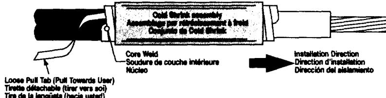
2. Make connection and clean cable insulation 2" (5 cm) minimum.
