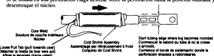
4. Pull loose pull tab gently while unwinding in a counter-clockwise direction.
