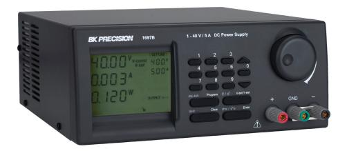
The 1696B Series of compact 200 W DC power supplies are equipped with programming and protection features commonly found in more expensive performance instruments. Programming features include list mode for repetitive operation and 10 user-configurable voltage/current presets for quick recall. These benchtop power supplies also support adjustable voltage and current limits to protect the device under test.
