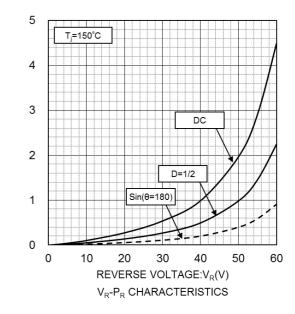
REVERSE POWER DISSIPATION:P<sub>R</sub>(W)
