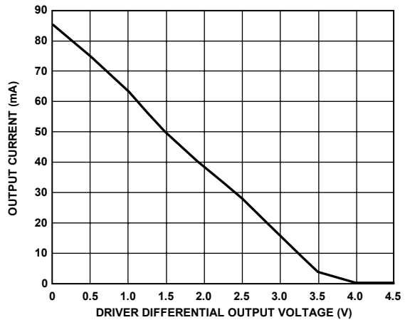
Figure 7. Output Current vs. Driver Differential Output Voltage
