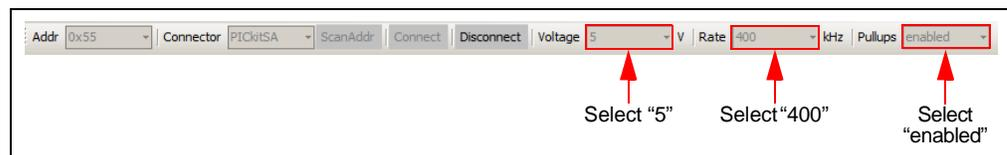
**FIGURE 4-1:** Connection Bar.
