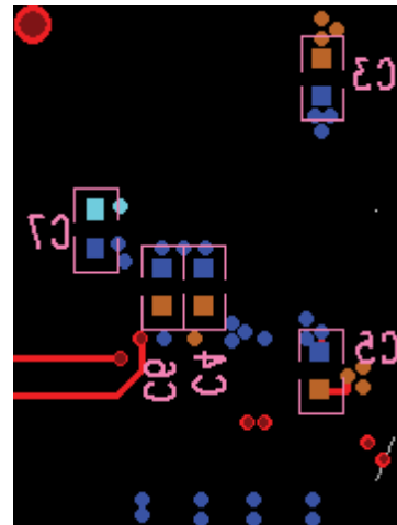
Figure 63. Bottom Layer Decoupling
