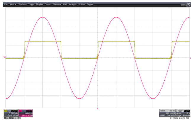
Figure 13 – 230 VAC 50 Hz. CH1: ZCD, 5 V / div., 5 ms / div. CH2: V_{IN} , 100 V / div., 5 ms / div.
