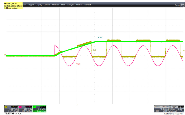
Figure 19 – 120 VAC 60 Hz, Full Load. CH1: ZCD, 5 V / div., 5 ms / div. CH2: V_{IN} , 100 V / div., 5 ms / div. CH4: V_{OUT} , 5 V / div., 5 ms / div.
