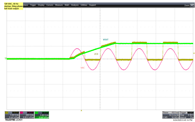
Figure 15 – 120 VAC 60 Hz, Full Load. CH1: ZCD, 5 V / div., 5 ms / div. CH2: V IN , 100 V / div., 5 ms / div. CH4: V OUT , 5 V / div., 5 ms / div.
