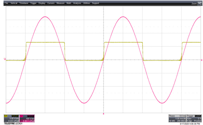
Figure 11 – 230 VAC 50 Hz. CH1: ZCD, 5 V / div., 5 ms / div. CH2: V_{IN} , 100 V / div., 5 ms / div.
