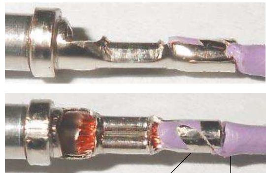
Skewing of Wire Insulation Acceptable Slight Deformation of Wire Insulation Acceptable
