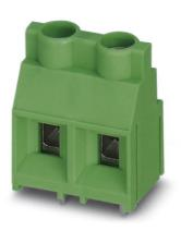
PCB terminal block, nominal current: 32 A, rated voltage: 690 V, pitch: 9.5 mm, no. of positions: 2, mounting: Soldering, type of connection: Screw connection, connection direction from the conductor to the PCB:  $0^{\circ}$
