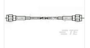
TE Part #1337808-1 50 OHM COAX SMA STR PLUG STR P
