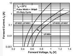
Figure 2. Forward Characteristics
