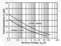
Figure 5. Typical Junction Capacitance
