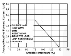
Figure 1. Forward Current Derating Curve
