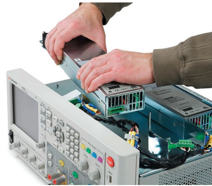
Figure 1. DC power modules are easily installed into the N6705 DC power analyzer mainframe.
