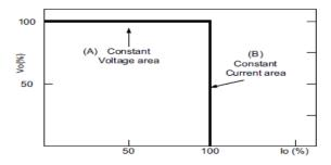
Typical LED power supply I-V curve
