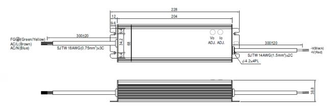
※ IP65 rated. Output voltage and constant current level can be adjusted through internal potential meter. (Can access by removing the rubber stopper on the case.)
