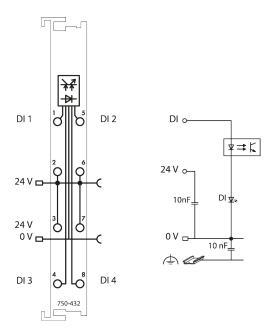
Figure 5: Circuit Diagram
