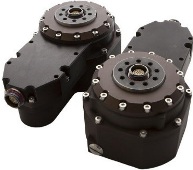
Servo drives designed around Servosila SC-25C brushless/brushed motor controllers
