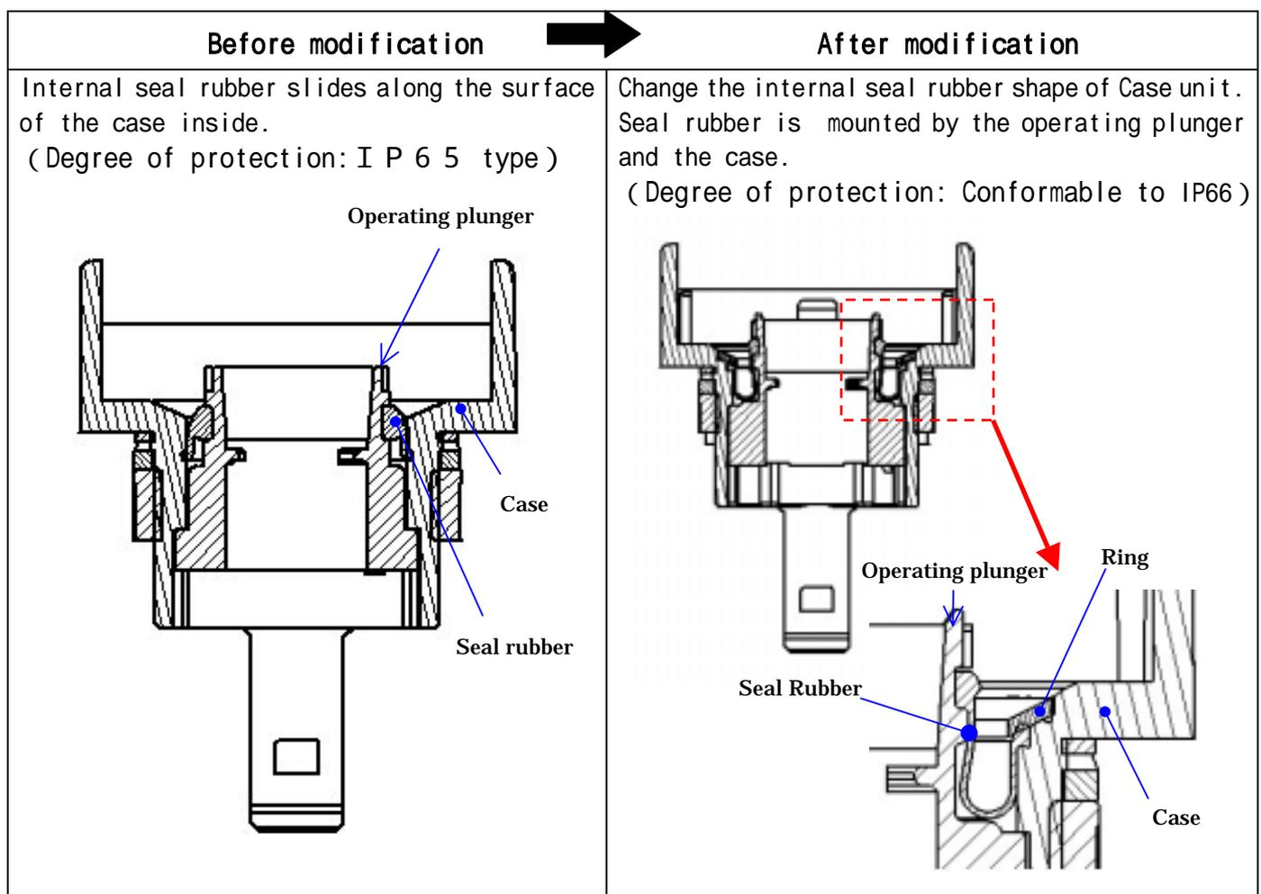
**Change of Pushbutton unit (For I P 6 5 type only - Not include I P 4 0 type)**
