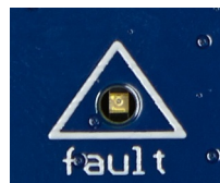
Figure 6-10. Fault LED, used to Indicate the Status of the Analog Sampling Circuitry
