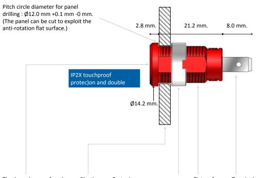
The 4 mm banana female connection complies with the 4 mm banana plugs of most of the worldwide most famous manufacturers and meets the requirements of interchangeability dimensions of the French standard NF C 93-440:1986.
