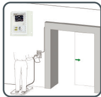
Connection with door access system
