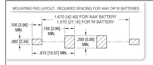
THIS DOCUMENT IS THE PROPERTY OF KEYSTONE ELECTRONICS CORP. AND SHALL NOT BE REPRODUCED, DISTRIBUTED OR USED AS A BASIS FOR MANUFACTURE WITHOUT PRIOR WRITTEN PERMISSION FROM KEYSTONE ELECTRONICS CORP.
