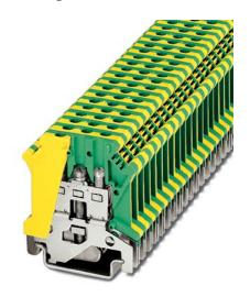
Ground terminal block with screw connection, cross section: 0.2 - 4 mm2, AWG: 24 - 12, width: 6.2 mm, color: Green-yellow
