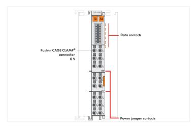
This potential multiplication module provides 0 V to the outputs in combination with the 750-1504 16-Channel Output Module (also suitable for 8-channel output modules with a single wire connection).
