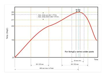
Fig 2. Infrared soldering profile
