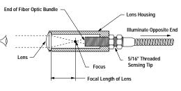
Lenses are most efficient when they are located slightly beyond their focal length distance from the sensing end of the fiber optic bundle. The easiest way to focus a lens is to treat it like a magnifying glass.
