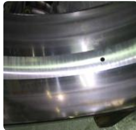
Outer ring raceways of spherical roller bearing showing abrasive wear
