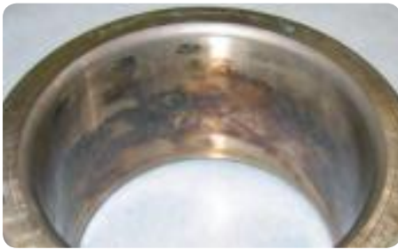
Fretting corrosion in the bore of bearings, resulting from inadequate shaft fit
