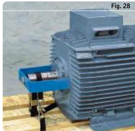
Lock the shaft and the bearings before transport
