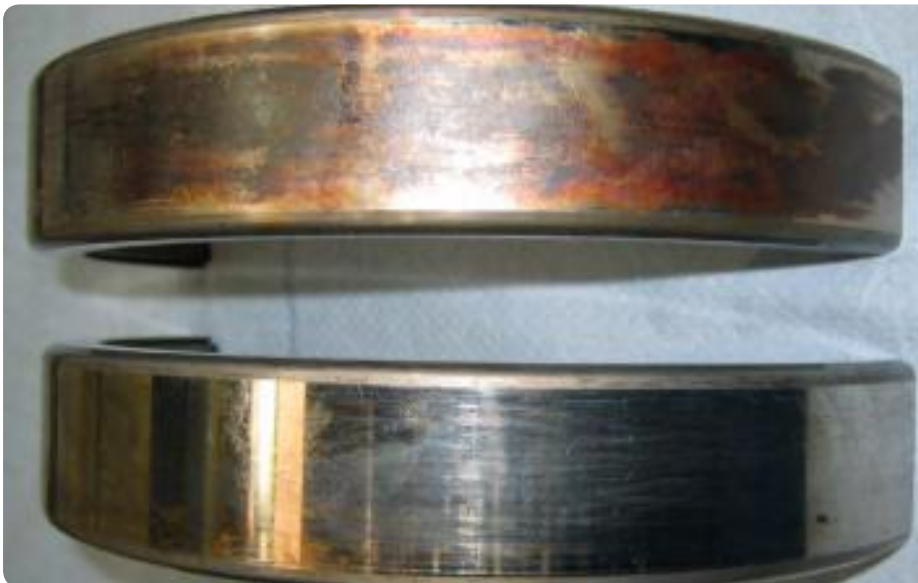
Fretting corrosion on the outer diameter of a bearing
