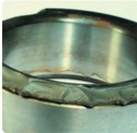
Forced fracture Cracked flanges of a cylindrical roller bearing inner ring due to impact load
