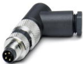
Connector, 4-position, Plug angled M8, A-coded, Screw connection, Knurl material: Nickel-plated brass, External cable diameter 3.5 mm ... 5 mm
