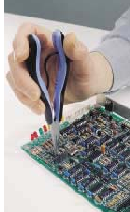
The Rx7890 in an inverted grip is used to straighten a connector pin. See page 48 for more on Rx7890.
