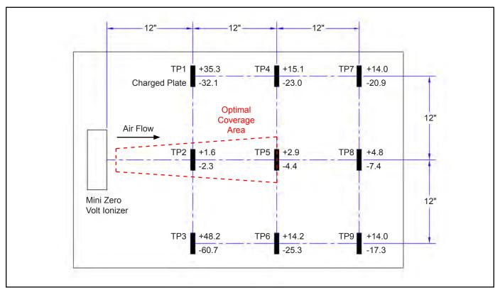
Figure 6. Neutralization (Discharge) Times
