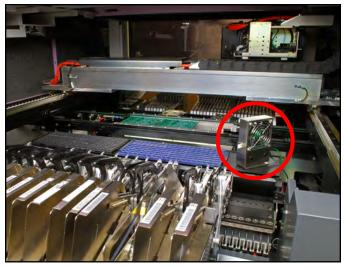
Figure 5. Using the Mini Zero Volt Ionizer 2 inside automated machinery.
