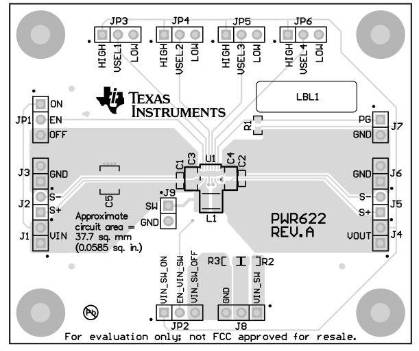
Figure 4-1. Assembly Layer
