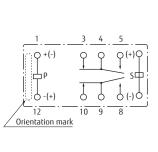
PC board mounting hole layout (BOTTOM VIEW)
