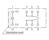
PC board mounting hole layout (BOTTOM VIEW)
