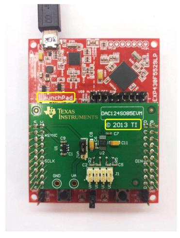
Figure 7. DAC124S085EVM Attached to MSP430
