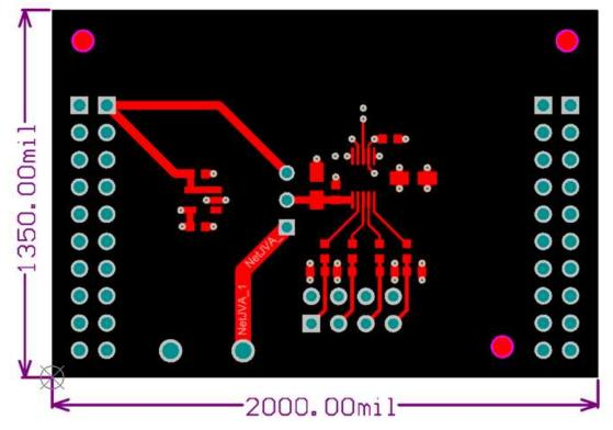
Figure 11. Top Layer Routing
