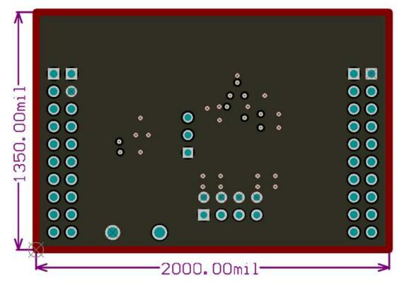
Figure 13. Ground Layer Routing
