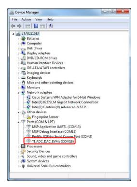
Figure 6. Driver Installed
