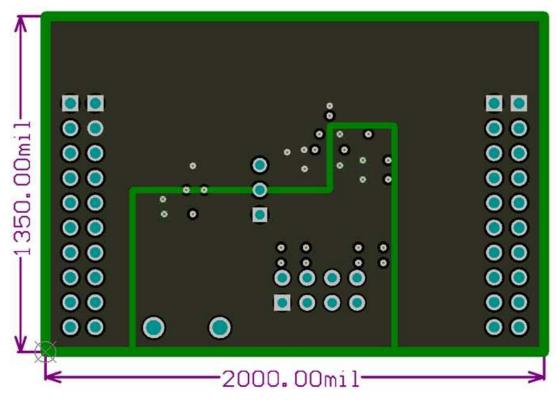
Figure 12. Power Layer Routing
