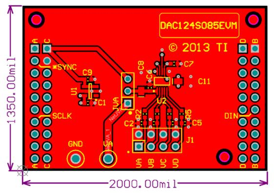
Figure 10. Top Assembly Layer
