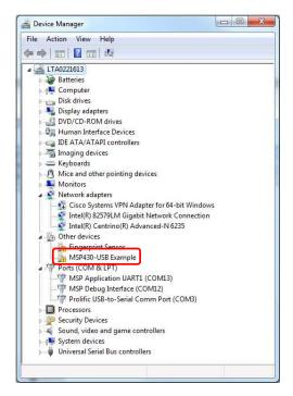
Figure 4. Driver Not Installed
