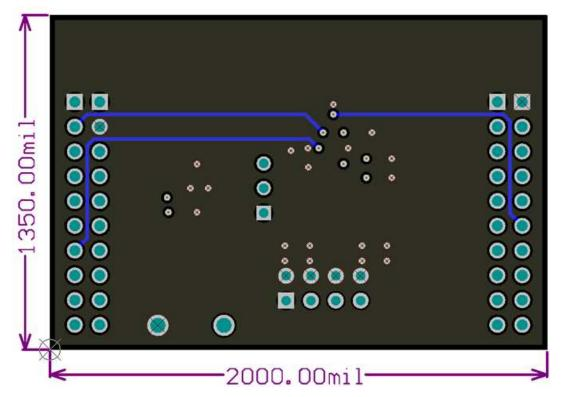
Figure 14. Bottom Layer Routing
