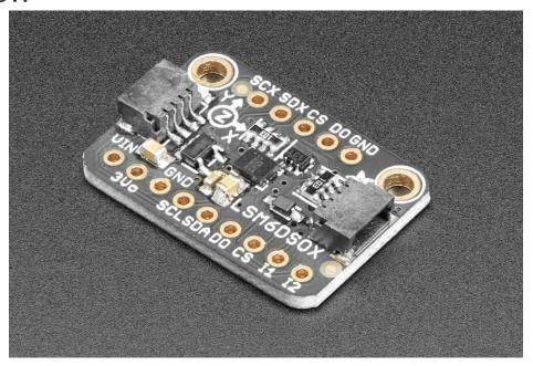
Behold, the ST LSM6DSOX: The latest in a long line of quality Accelerometer+Gyroscope 6-DOF IMUs from ST. Along with the LSM6DSOX, this guide will cover the *industrial* version, the ISM330DHCX and their wider range sibling the LSM6DSO32. All are pin-compatible and are nearly code-compatible - we'll be using the same library code and wiring diagrams to connect to both
