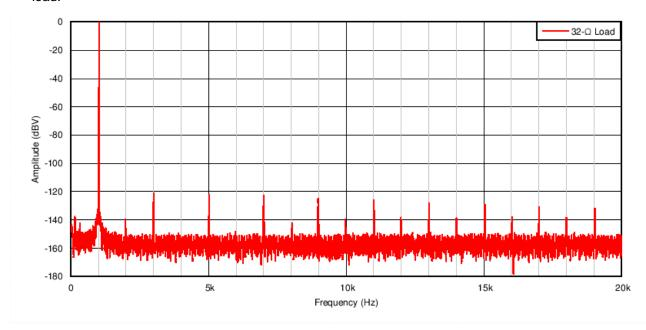
Figure 5. FFT With a 32- $\Omega$  Load
