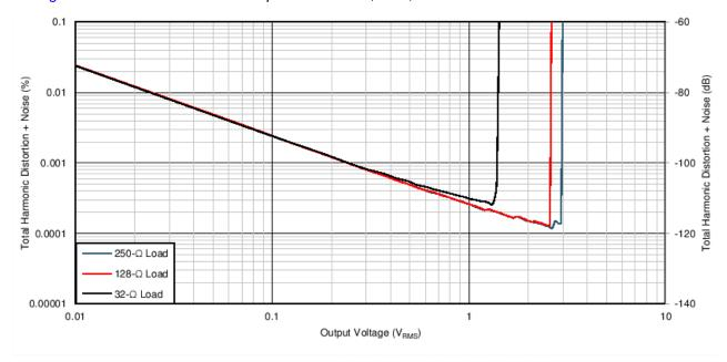
Figure 4. THD+N vs. Amplitude for a 32-, 128-, and 250- $\Omega$  Load
