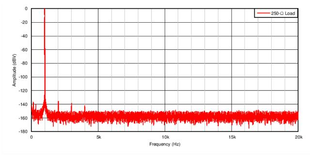
Figure 7. FFT With a 250- $\Omega$  Load
