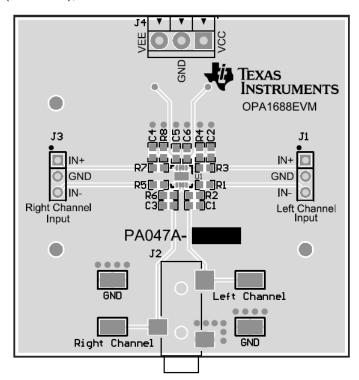
Figure 8. Top Layer PCB Layout
