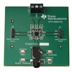
This user's guide contains information for the OPA1688 as well as support documentation for the OPA1688 evaluation module (EVM). Included are the performance specifications, set-up procedure, modifications, measured data, printed circuit board (PCB) layout, schematic, and bill of materials (BOM) of the OPA1688EVM.
