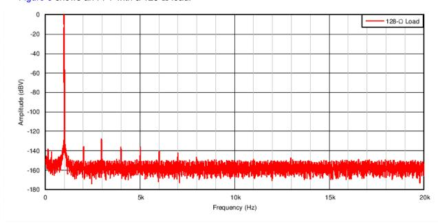
Figure 6. FFT With a 128-Ω Load
