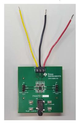
Figure 2. Power Supply Connections
