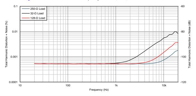
Figure 3. THD+N vs. Frequency for a 32-, 128-, and 250-Ω Load
