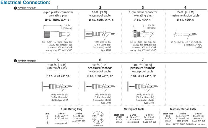
\*-Test pressure: 100 feet [30 meters] H<sub>2</sub>O (40 PSID) Test Medium: Air; Duration: 2 hours. \*\* - applies to stainless steel enclosure only. \*\*\*14-32 VDC for hazardous area option.
