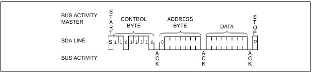
FIGURE 6-2: SRAM/RTCC SEQUENTIAL WRITE
