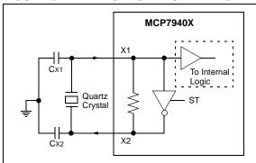
Note 1: The ST bit must be set to enable the crystal oscillator circuit.
