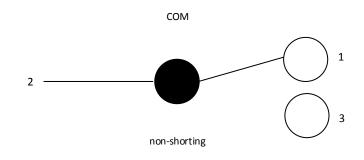
Type of Schematic: SPDT
