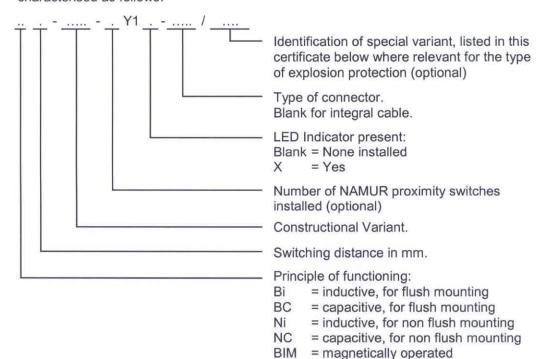
The range of Two Wire Proximity Sensors ...-..../ .... consists of various constructional variants classified into ten Type Groups.
