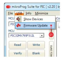
Connect your mikroProg™ programmer and debugger with your PC via USB cable. If drivers are correctly installed USB Link amber colored LED will turn on. Start your mikroProg Suite™ for PIC® v2.20 software. Under **USB menu** click the "Firmware Update" option in order to start. If you have older versions of the software installed, make sure to download and install the latest version from the mikroElektronika website (www.mikroe.com).
