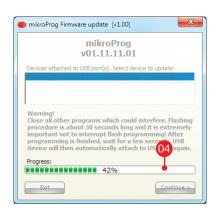
Firmware upgrade will start and progress bar will show the upgrade progress. The whole process takes about 30 seconds. While firmware update is in progress DO NOT DISCONNECT USB CABLE from mikroProg<sup>™</sup> and **DO NOT START ANOTHER INSTANCE OF mikroProg** Suite<sup>™</sup> for PIC® SOFTWARE.
