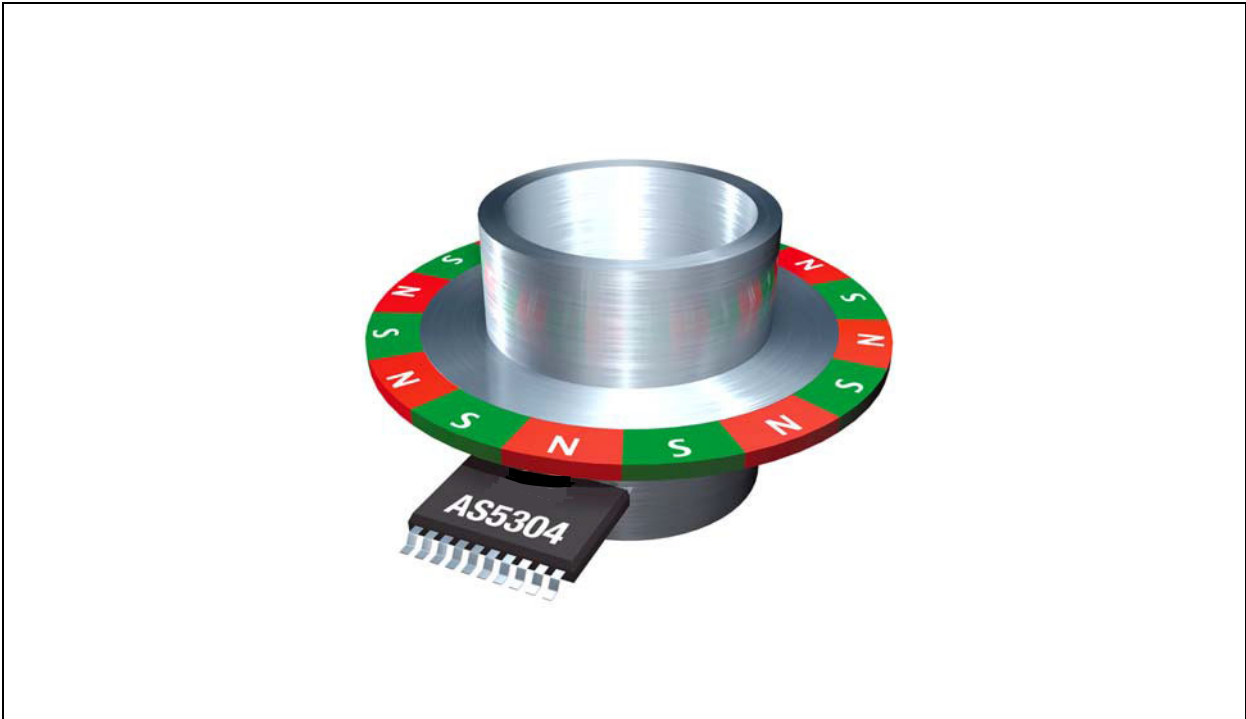
Figure 20: AS5304 (AS5306) with Multi-Pole Ring Magnet
