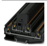
Fuse modular terminal block, Connection method: Push-in connection, Cross section: 0.2 mm²- 6 mm², AWG: 24 - 10, Nominal current: 6.3 A, Nominal voltage: 500 V, Width: 6.2 mm, Fuse type: G / 5 x 20, Fuse type: Glass / ceramics / ..., Mounting type: NS 35/7,5, NS 35/15, Color: black
