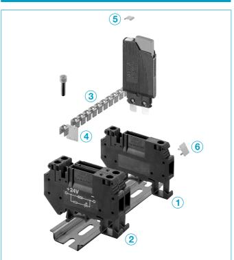
Terminal block for DIN rail mounting, with screw terminals up to 6 mm<sup>2</sup> cord, width 8.2 mm, dimensions 64x42.5x8.2 mm, headroom over the upper rail edge with circuit breaker fitted (OFF position) 84 mm.
