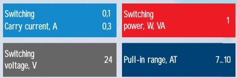
Any DC combination of V&A not to exceed the Switching power.
