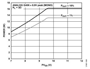
Figure 68. Power vs. PV<sub>DD</sub>, Analog Gain = 8.9 V peak,  $R_L$  = 3  $\Omega$
