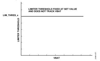
Figure 76. Limiter Fixed (LIM\_EN\_x = 0b01, VBAT\_TRACK\_x = 0b0)
