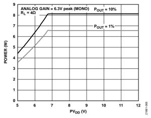
Figure 67. Power vs. PV<sub>DD</sub>, Analog Gain = 6.3 V peak,  $R_L$  = 4  $\Omega$
