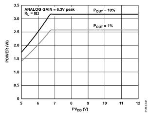
Figure 43. Power vs. PV<sub>DD</sub>, Analog Gain = 6.3 V peak,  $R_L = 8 \Omega$
