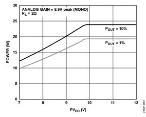
Figure 64. Power vs. PV<sub>DD</sub>, Analog Gain = 8.9 V peak,  $R_L$  = 2  $\Omega$
