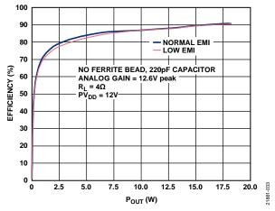
Figure 35. Efficiency vs.  $P_{OUT}$ , No Ferrite Bead, Analog Gain = 12.6 V peak,  $R_L = 4 \Omega$ ,  $PV_{DD} = 12 V$
