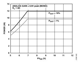
Figure 63. Power vs. PV<sub>DD</sub>, Analog Gain = 8.9 V peak,  $R_L$  = 4  $\Omega$
