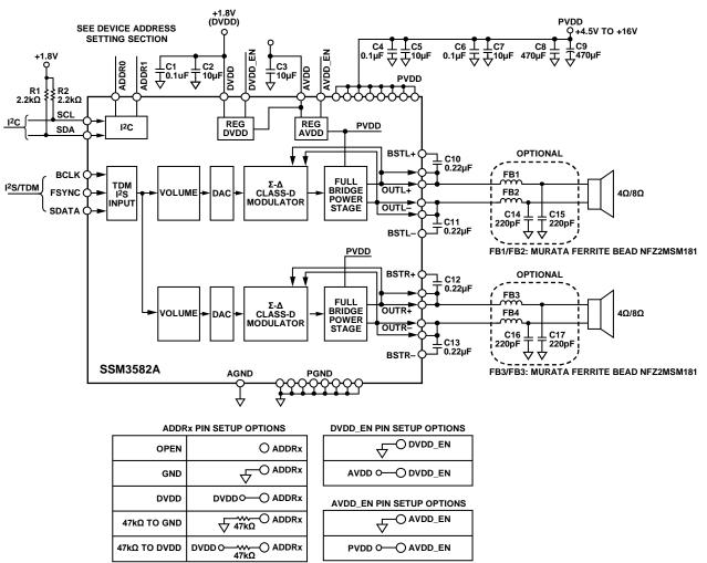
Figure 86. Typical Application Circuit for Stereo Output
