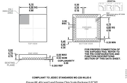
Figure 88. 40-Lead Lead Frame Chip Scale Package [LFCSP] 6 mm × 6 mm Body and 0.75 mm Package Height (CP-40-7) Dimensions shown in millimeters
