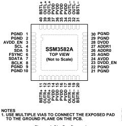
Figure 6. Pin Configuration
