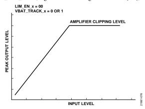
Figure 77. Limiter Example (LIM\_EN\_x = 00, VBAT\_TRACK\_x = 0 or 1)
