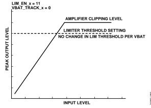
Figure 80. Limiter Example (LIM\_EN\_x = 11, VBAT\_TRACK\_x = 0)
