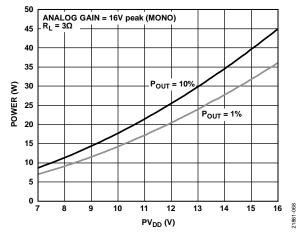
Figure 70. Power vs. PV<sub>DD</sub>, Analog Gain = 16 V peak,  $R_L = 3 \Omega$
