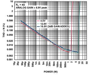
Figure 22. THD + N vs. Power,  $R_L = 4 \Omega$ , Analog Gain = 8.9 V peak
