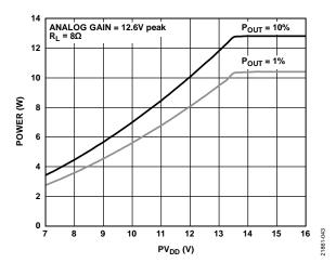
Figure 45. Power vs. PV<sub>DD</sub>, Analog Gain = 12.6 V peak,  $R_L = 8 \Omega$
