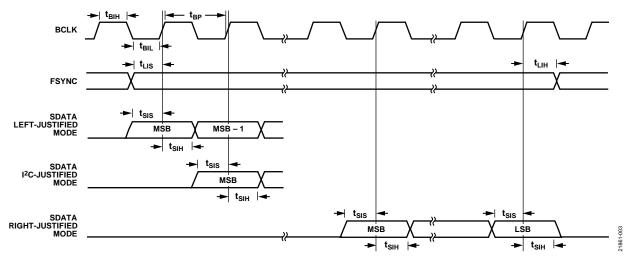
Figure 3. Serial Input Port Timing
