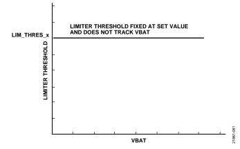
Figure 81. Limiter Fixed (LIM\_EN\_x = 11, VBAT\_TRACK\_x = 0)
