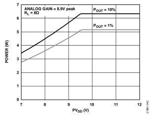
Figure 44. Power vs. PV<sub>DD</sub>, Analog Gain = 8.9 V peak,  $R_L$  = 8  $\Omega$
