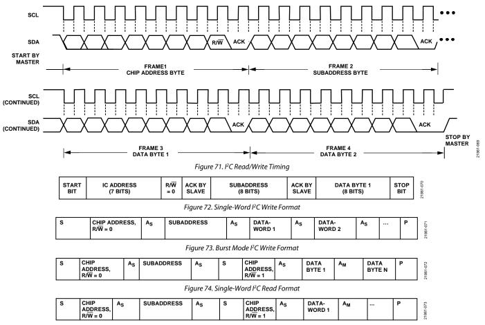
Figure 75. Burst Mode I<sup>2</sup>C Read Format
