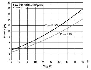
Figure 46. Power vs. PV<sub>DD</sub>, Analog Gain = 16 V peak,  $R_L = 8 \Omega$
