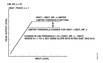
Figure 78. Limiter Fixed (LIM\_EN\_x = 01, VBAT\_TRACK\_x = 1)
