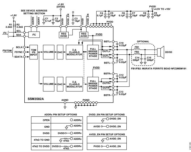
Figure 87. Typical Application Circuit for Mono Output
