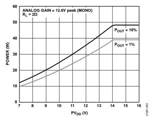
Figure 65. Power vs. PV<sub>DD</sub>, Analog Gain = 12.6 V peak,  $R_L = 2 \Omega$
