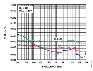
Figure 17. THD + N vs. Frequency,  $R_L = 4 \Omega$ ,  $PV_{DD} = 16 V$
