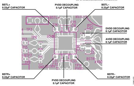
Figure 85. Recommended Component Placement
