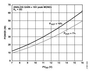
Figure 66. Power vs. PV<sub>DD</sub>, Analog Gain = 16 V peak,  $R_L = 2 \Omega$
