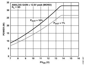
Figure 69. Power vs. PV<sub>DD</sub>, Analog Gain = 12.6 V peak,  $R_L$  = 3  $\Omega$
