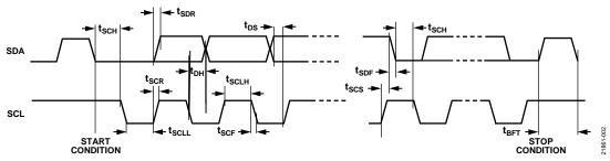
Figure 2. I<sup>2</sup>C Port Timing
