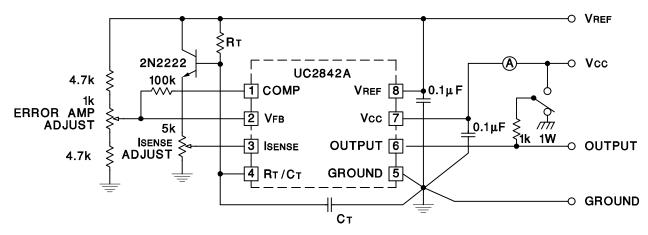
High peak currents associated with capacitive loads necessitate careful grounding techniques. Timing and bypass capacitors should be connected close to pin 5 in a single point ground. The transistor and 5k potentiometer are used to sample the oscillator waveform and apply an adjustable ramp to pin 3.
