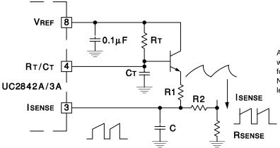
A fraction of the oscillator ramp can be resistively summed with the current sense signal to provide slope compensation for converters requiring duty cycles over 50%.
