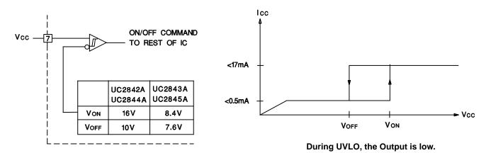
Figure 2. Under Voltage Lockout
