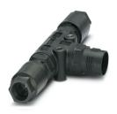
QUICKON T-distributor, black, 4+PE-pos., 1.0  $\rm mm^2$  ... 2.5  $\rm mm^2/690$  V/20 A, for cable diameter of 6 mm ... 11 mm, with two QUICKON nuts
