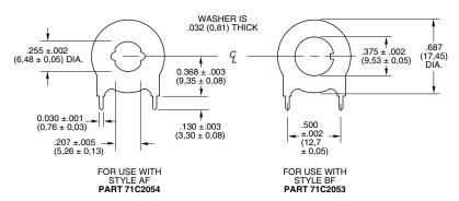
For printed circuit styles. Mounting bushing provides additional support for the front end of the switch. Order separately by appropriate part number. Rotary switch discount applies.
