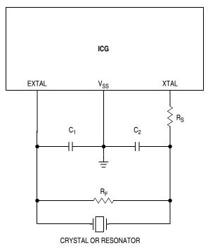
Figure 7-5. External Frequency Reference Connection
