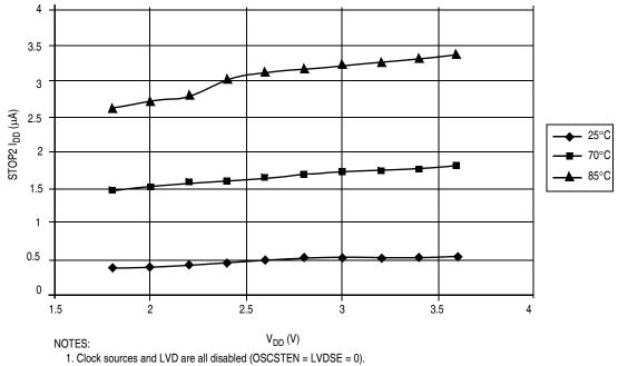
2. All I/O are set as outputs and driven to  $\dot{V}_{SS}$  with no load.
