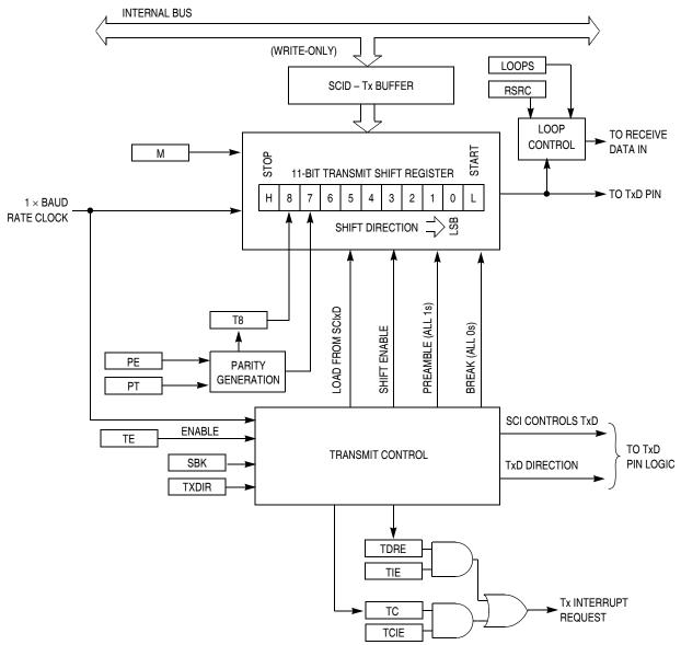
Figure 11-2. SCI Transmitter Block Diagram
