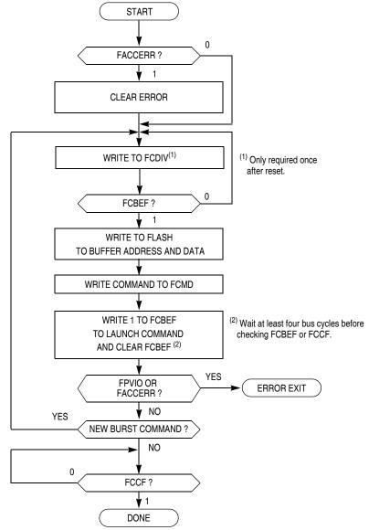
Figure 4-3. Flash Burst Program Flowchart
