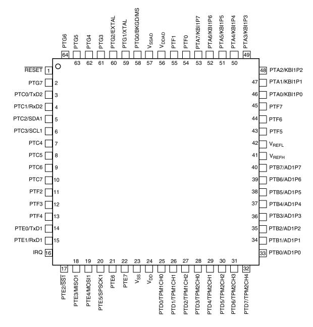
Figure 2-1. MC9S08GBxxA in 64-Pin LQFP Package
