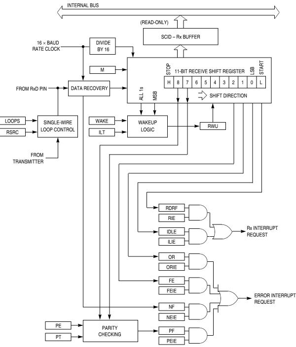
Figure 11-3. SCI Receiver Block Diagram
