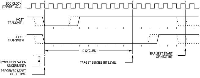
Figure 15-2. BDC Host-to-Target Serial Bit Timing
