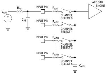
Figure 14-3. Resistor and Capacitor Placement
