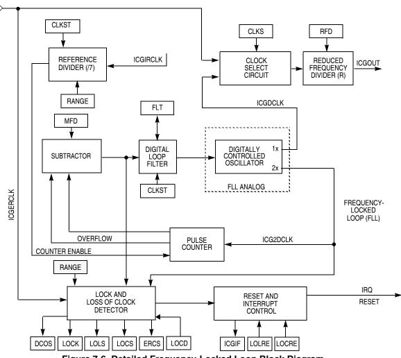
Figure 7-6. Detailed Frequency-Locked Loop Block Diagram
