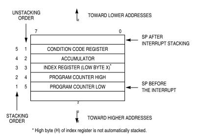
Figure 5-1. Interrupt Stack Frame
