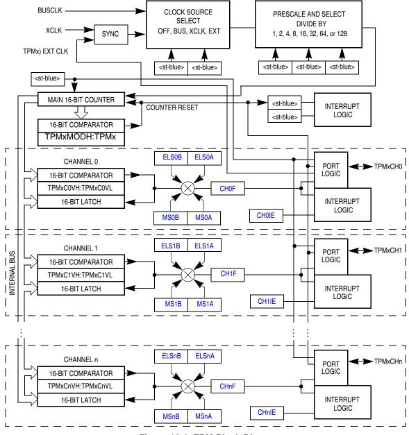
Figure 10-2. TPM Block Diagram
