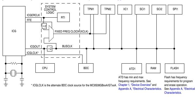
Figure 7-1. System Clock Distribution Diagram
