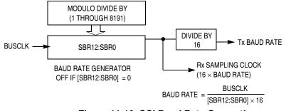
Figure 11-12. SCI Baud Rate Generation
