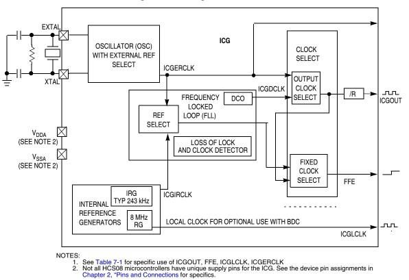
Figure 7-3. ICG Block Diagram
