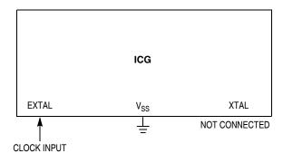
Figure 7-4. External Clock Connections
