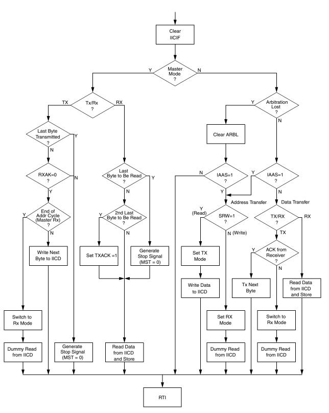
Figure 13-11. Typical IIC Interrupt Routine
