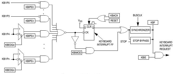
Figure 9-3. KBI Block Diagram
