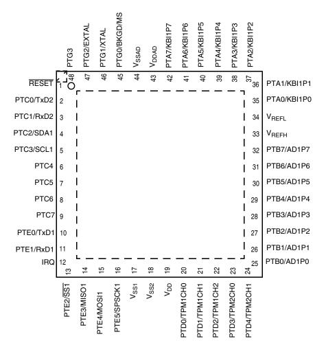
Figure 2-2. MC9S08GTxxA in 48-Pin QFN Package
