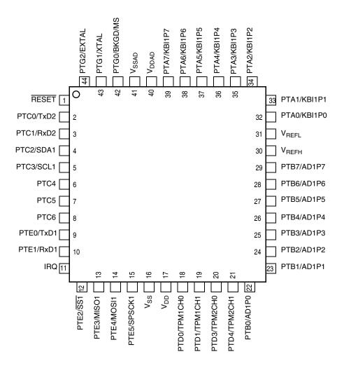
Figure 2-3. MC9S08GTxxA in 44-Pin QFP Package
