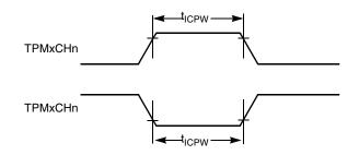
Figure A-15. Timer Input Capture Pulse
