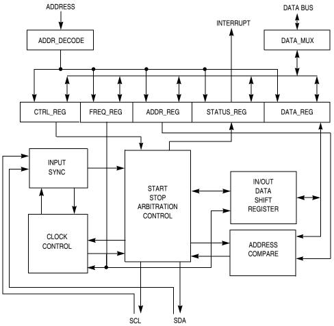
Figure 13-2. IIC Functional Block Diagram
