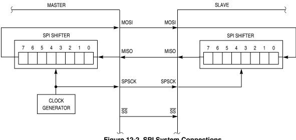
Figure 12-2. SPI System Connections
