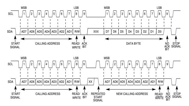
Figure 13-8. IIC Bus Transmission Signals
