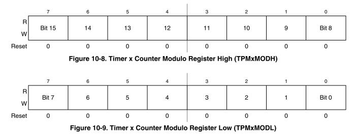
It is good practice to wait for an overflow interrupt so both bytes of the modulo register can be written well before a new overflow. An alternative approach is to reset the TPM counter before writing to the TPM modulo registers to avoid confusion about when the first counter overflow will occur.
