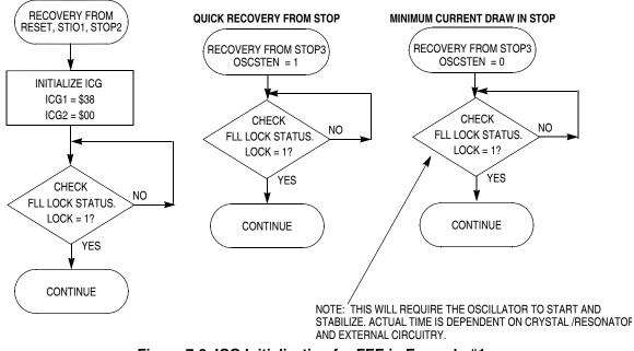
Figure 7-8 shows flow charts for three conditions requiring ICG initialization.
