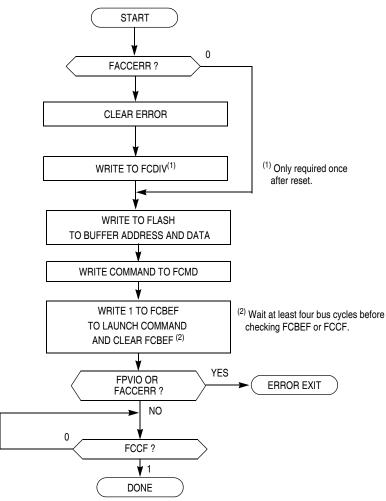
Figure 4-2. Flash Program and Erase Flowchart
