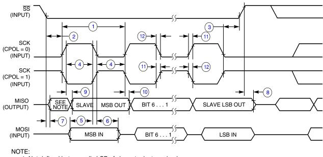
Figure A-18. SPI Slave Timing (CPHA = 0)
