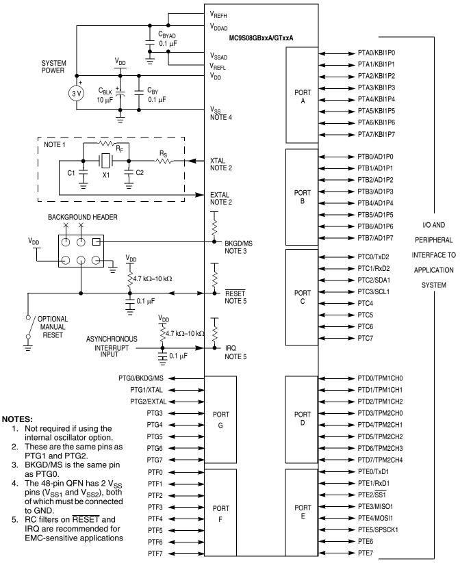
Figure 2-5. Basic System Connections
