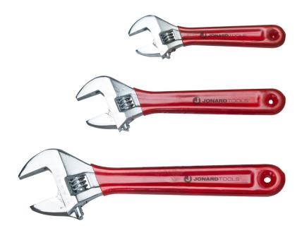
Jonard's adjustable wrenches are made of chrome vanadium steel with a chrome plated finish. They are forged and heat treated for maximum strength. Handles are covered with a red vinyl grip for user comfort. The knurled worm gear is precision formed and the operation is smooth and trouble free. For acurate and faster adjustments use the metric or English scales on either side of the jaws. With extra wide jaws, a smaller wrench works on bigger jobs. Great for tight spaces.
